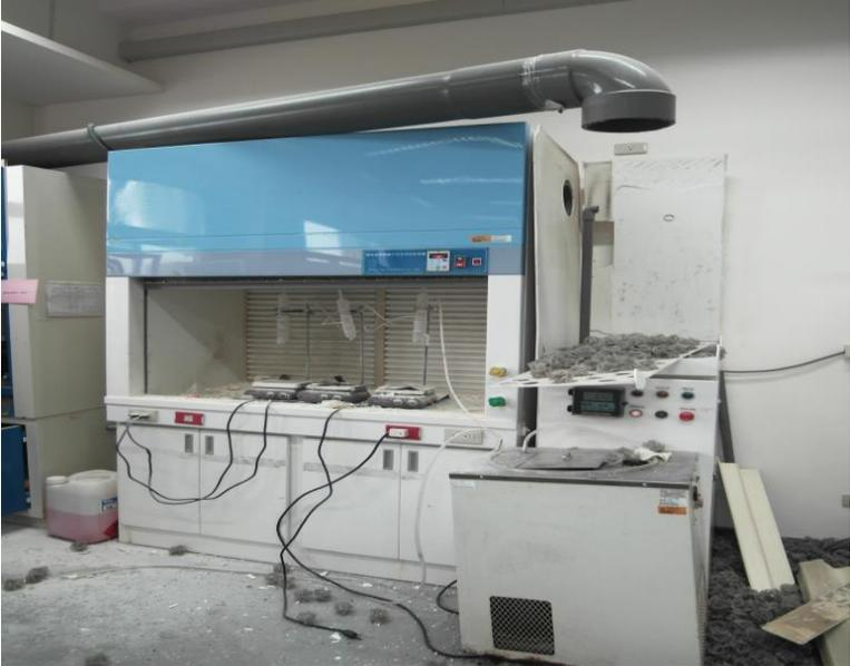
A photograph of a laboratory fume hood and an air purifier. The fume hood has a blue top and a white front. The glass front is broken and hanging off. A large black duct is attached to the top. The air purifier is a white unit with a control panel and a filter. The floor is covered in debris, including broken glass and dust.                               | <p>圖 2 為事故現場排煙櫃玻璃、導管及水洗式廢氣清淨裝置本體已經破損、脫落。</p>                                                                                     |
